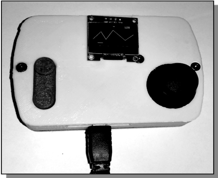
A printed Arduino / NodeMCU based development platform. SPI and I2C displays are supported; shown here with an 0.96" OLED, analog joystick and 2 menu buttons. (Photo by author)
