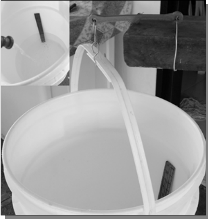
Test setup and inset of using the calibrated measuring stick (Photo by author)
