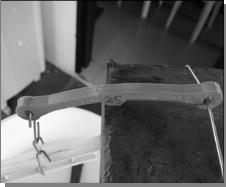
25% infill load beam under test. Note the stress lines forming on the upper surface, and significant bending. (Photo by author)
