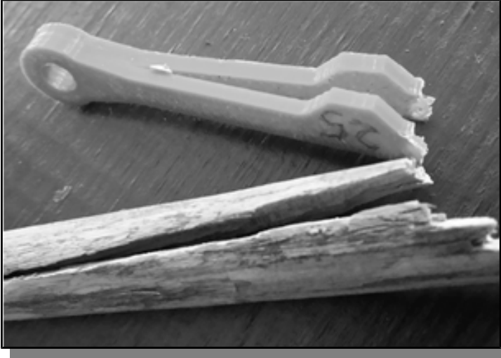
Photo showing a printed sample and a wooden twig split along the direction of their “grain”. (Photo by author)
