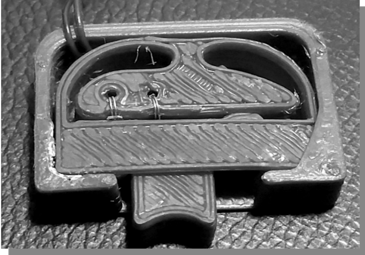
The printed switch modeled in the previous illustrations, printed 15-mm wide. Note the wire wrapped through the holes and the spring holding the contact assembly against the slider. (Photo by author)
